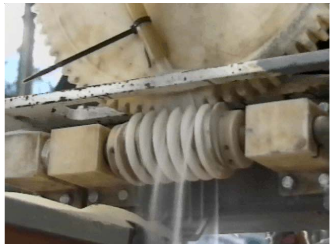
figure 5: durability test of worm gear
