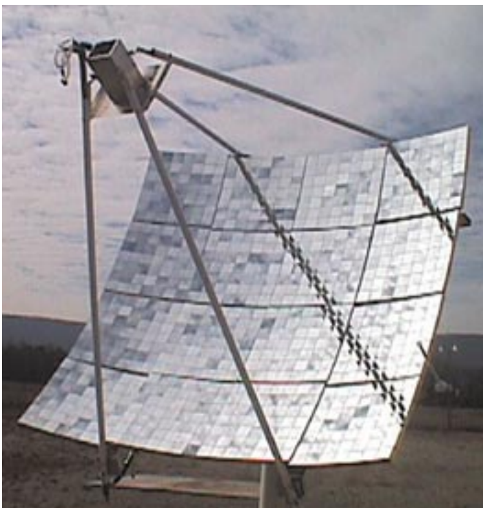
This small photovoltaic solar dish conversion system is being developed by Concentrating Technologies, LLC.
