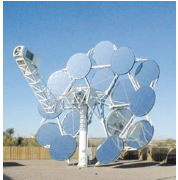
This Science Application International Corporation/ STM Power Inc. 25 kW Dish-Stirling System is operating at a Salt River Project site in Phoenix, AZ.
