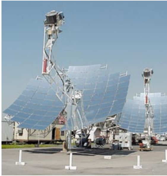
The Boeing/Stirling Energy Systems DECC project will evaluate the performance of the "critical" parts of the Stirling engine and develop the next-generation of the 25 kW Dish-Stirling System.
